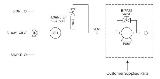
Figure 3-3: Piping Diagram for Vacuum Service Option
